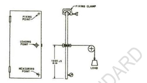
Figure 7 — Mounting of door shutter of buckling resistance test
