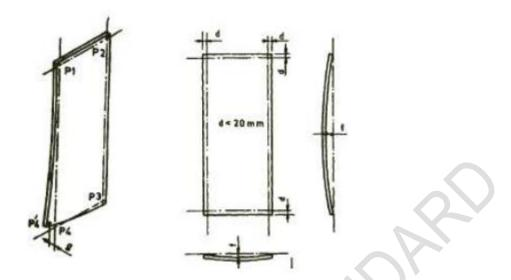
The reference plane is defined by the three points P1, P2, and P3, P4, is also situated on this plane. The measurement of the distance P4-P4, (g) gives the value of twist.
