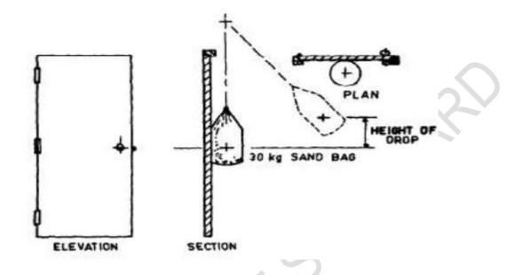
Figure 6 — Test arrangement for resistance to soft and light body impact
