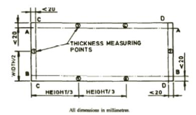
Figure 1 — Measurement of Dimensions
