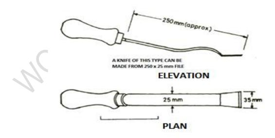
Figure 10 — Knife for testing plywood for adhesive of plies
